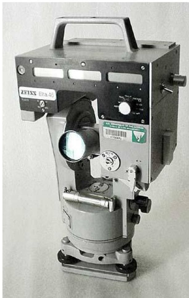
Figure 1.5 A Zeiss Elta 46 Total Station. (Photo Courtesy of National Museum of American History)
