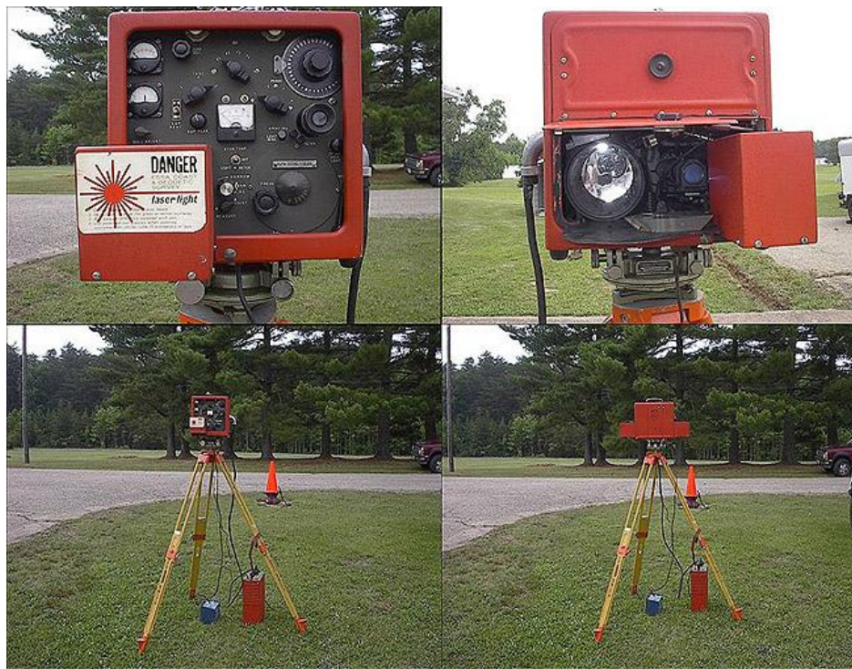
Figure 1.3 The "Big Red", a modified Geodimeter with Laser. Clockwise from top left: Control panel; optics; set up showing separate power packs for Geodimeter and laser; and a side view of the instrument. (From NOAA 200 Years Celebration Website, Photos courtesy of Charlie Glover)
