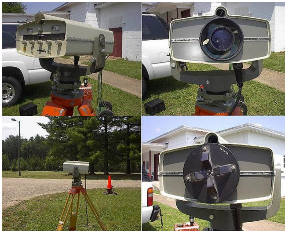
Figure 1.4 A HP Model 3800B Distance Meter. The cover shown on the bottom right is a calibration cap designed and built by the Instrument and Methodologies Branch of the National Geodetic Survey. (From NOAA 200 Years Celebration Website, Photos courtesy of Charlie Glover)
