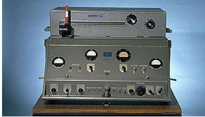
Figure 1.1 A circa 1959 AGA Geodimeter 2A showing the front control panel. (From NOAA 200 Years Celebration Website, Photos courtesy of the University of New South Wales School of Surveying and Spatial Information Systems Virtual Surveying Instrument Collection)
