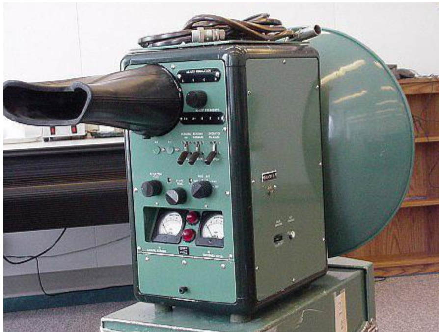
Figure 1.2 A Tellurometer (From NOAA 200 Years Celebration Website, Photos courtesy of the Alberta Land Surveyor's Association Surveying Instrument Collection)
